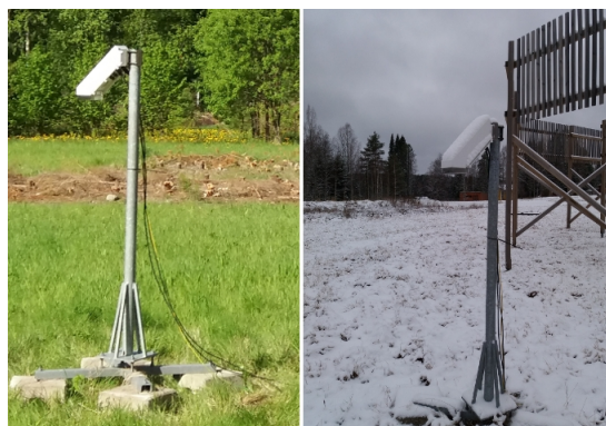
Fig. 4: Field mill installation: June 2017 (left) / November 2017 (right).
